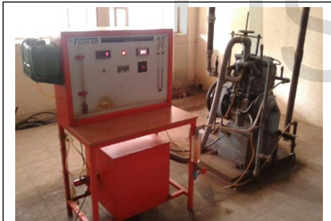
Fig. 1. Photograph of the experimental setup showing the test rig and the twin cylinder DI diesel engine.
